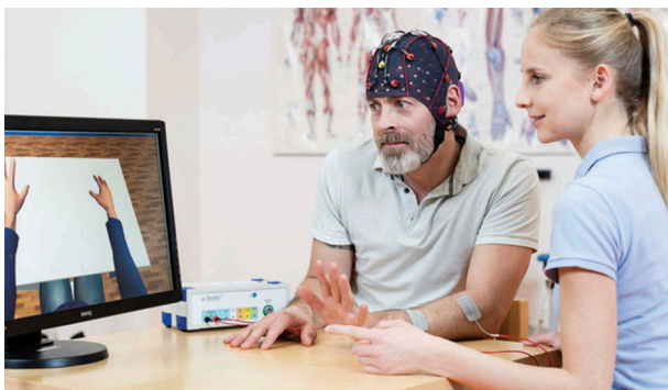
Figure 1. Components of the recoveriX system: computer screen with the 3D avatar in a first-person perspective, FES stimulator, EEG cap with active electrodes.
