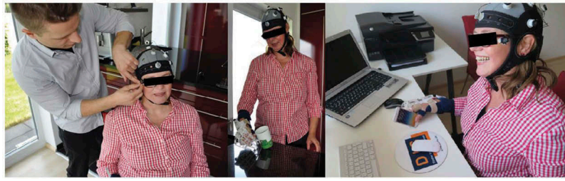
Figure 5. Illustration of the Tübingen hybrid brain/neural hand exoskeleton (B/NHE) for home-based stroke neurorehabilitation. The brain's electrical activity from the ipsilesional hemisphere is recorded and transmitted to a tablet computer detecting sensorimotor rhythm (SMR) desynchronization associated with the attempt to open the paralyzed fingers. Hand closing motions are either performed by the patient or (in case of flaccid paralysis) by horizontal eye movements detected by electrooculography (EOG). After specific training periods, in which B/NHE-supported hand opening and closing is learned, patients use the system in their daily-life environments to perform activities of daily living, fostering generalization of learned skills.
