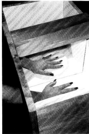
*Fig. 4-2 The Virtual Reality box created by Ramachandran et. al. [23]*
