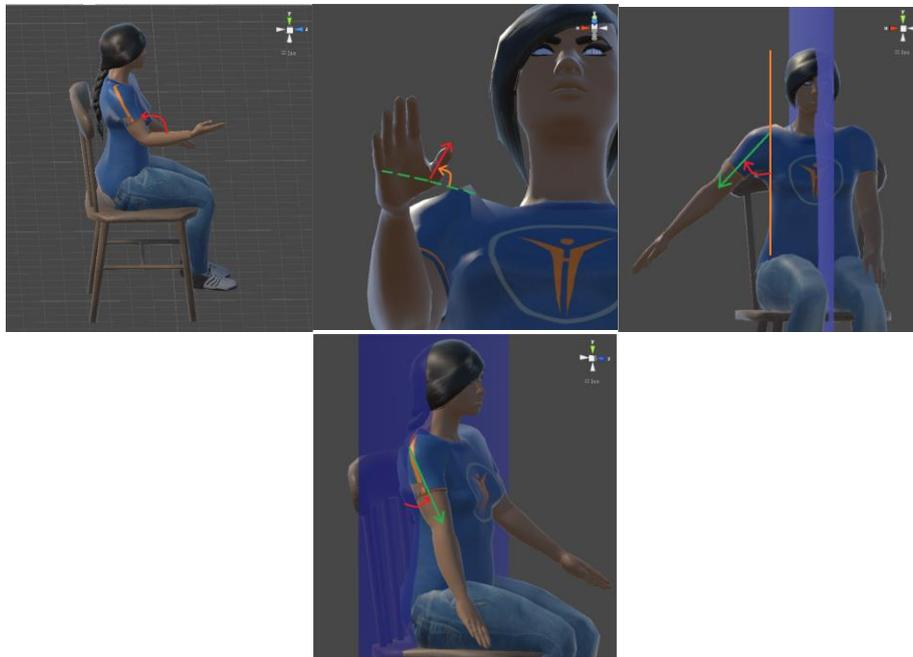
*Fig. 8-17 The angles considered for evaluating the movement score for Forearm Flexion-Extension, Thumb Opposition, Arm Adduction-Abduction, Arm Anteduction-Retroduction*
