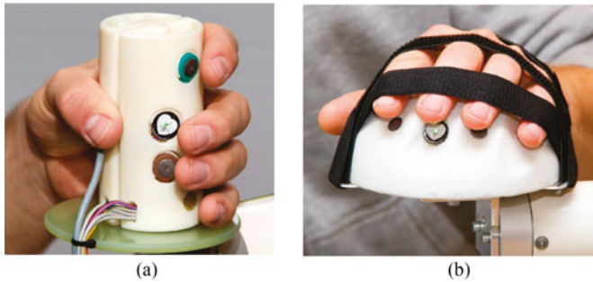
Fig. 2. Handle designs with integrated physiological sensors. (a) Cylindrical shape (c-handle). (b) Hemispherical shape (s-handle).
