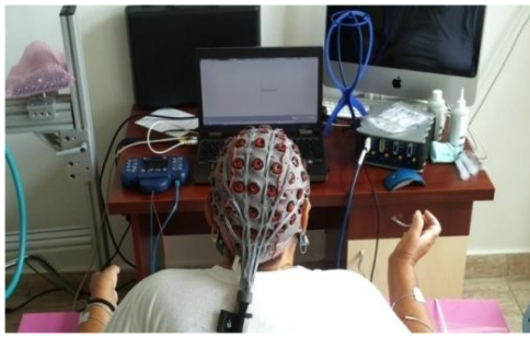
Figure 1. One training session with recoveriX. The patient has FES pads on the forearms, which are connected to an FES control system in the left side of the picture. The amplifier is shown on the right. The monitor shows an arrow extending to the right, reflecting that the patient is imagining right hand movement. Concordantly, the FES system is stimulating the right forearm, causing right wrist dorsiflexion.
