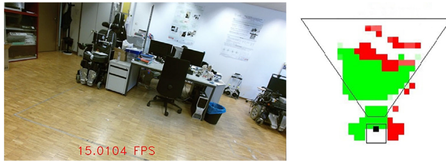
Fig. 4. Ground detection while the robot is walking. It can be seen that the tilt angle of the camera is high during the exoskeleton's locomotion which makes the problem more challenging.
