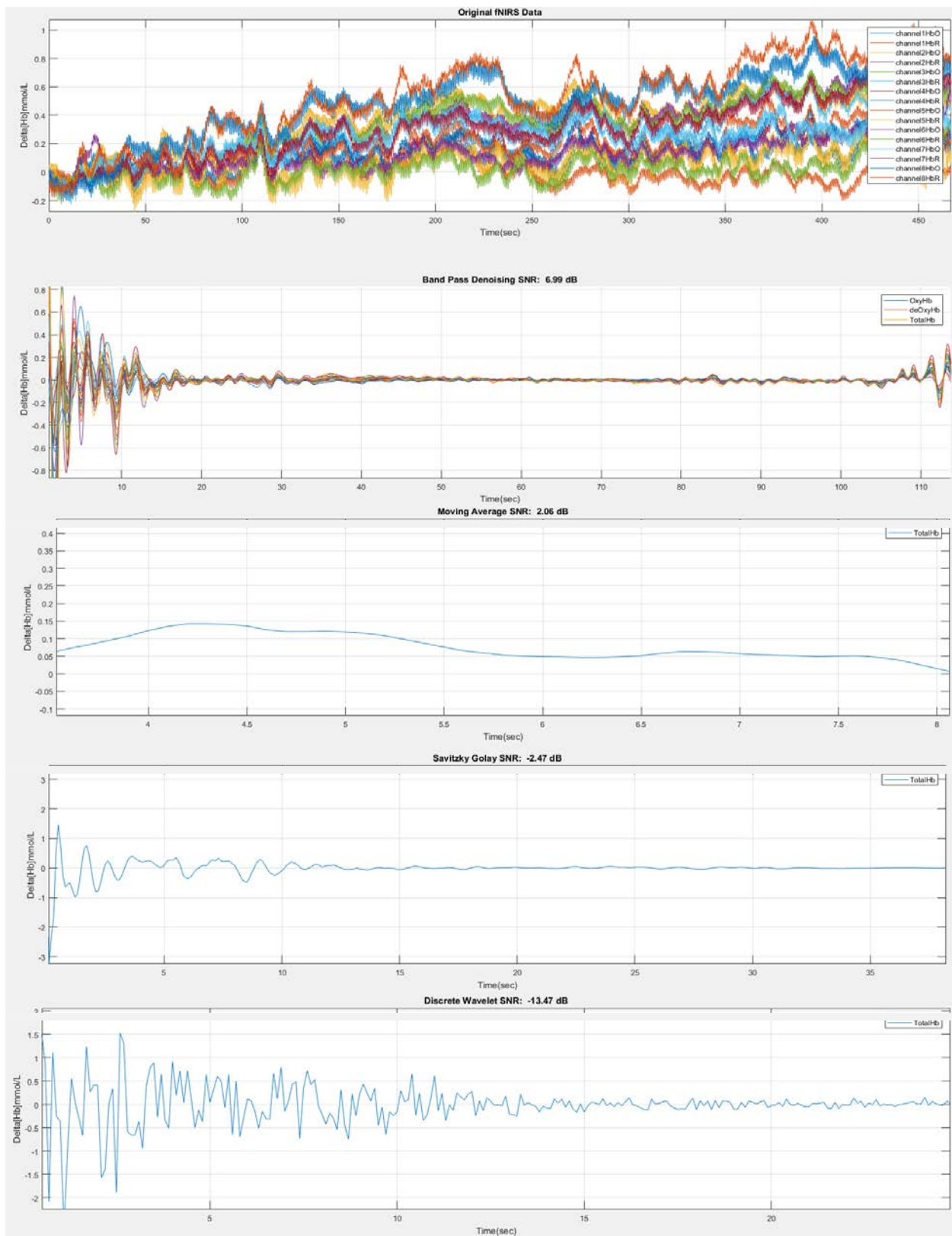
Figure 41. DCT detrending results for subject #1. Data has motion corrected and the SNR value for each filtered signal has extracted.
