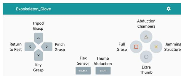
**FIGURE 5.** The smartphone app interface is used to control the exoskeleton glove operation. The user can combine the motions desired (e.g., full grasp with abducted fingers or tripod grasp with the extra thumb inflated and the jamming structures activated). The flex sensor can be selected to trigger the desired motion when a set bending angle is reached.
