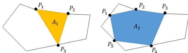
**FIGURE 9.** Illustration of the physical interpretation of the grasp quality measure based on the geometric relation between the object and the contact points for three contact points (left) and five contact points (right).  $P_1, P_2, P_3, \dots, P_n$  denote the contact points, and  $A_1$  and  $A_2$  denote the area generated by the contact points. The larger the area generated by the contact points the better the grasp.
