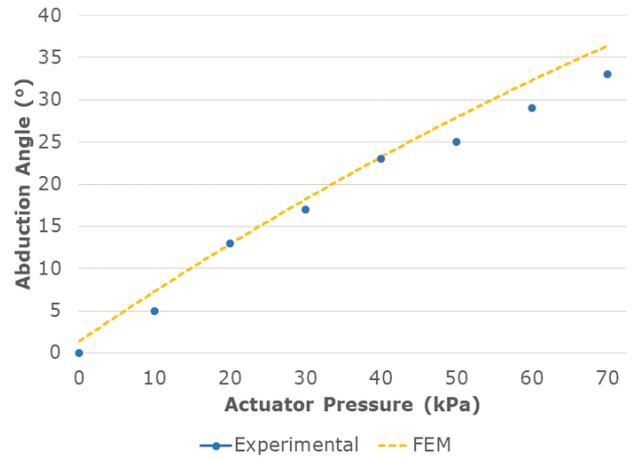
**FIGURE 7.** Abduction angles of the actuator obtained during the FEM analysis for multiple pressures compared to the experimentally measured abduction angles of the physical prototype. The results demonstrate a similar abducting behaviour for the model actuator and the actual soft actuator.
