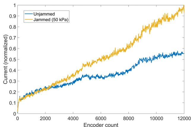
**FIGURE 12.** Motor current values while bending the finger. Two different conditions were used: index finger bending with the jamming structures activated (50 kPa) and deactivated (unjammed). The results show that when the structure is jammed, higher motor current is required to bend the finger.
