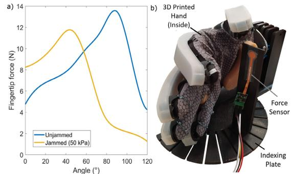
**FIGURE 10.** Results (subfigure a)) and experimental setup (subfigure b)) used for the fingertip force experiments conducted with the proposed exoskeleton glove under the jammed and unjammed control modes. The setup consists of a 3D printed hand (model hand) wearing the robotic glove, a force sensor, and an indexing plate with an increment value of 15°. The force profiles were acquired for a total of eight different positions (from 0° to 120°).
