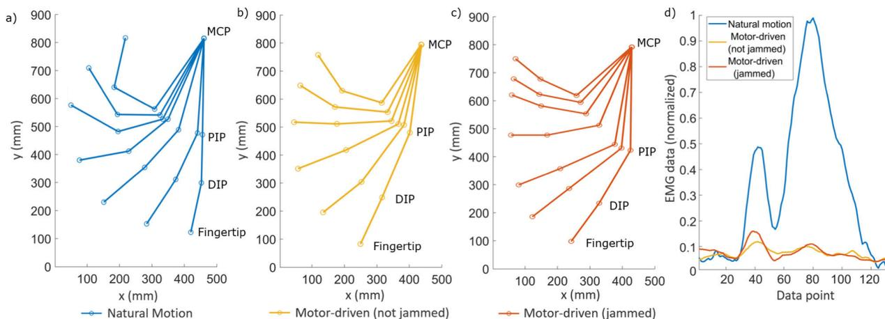
**FIGURE 11.** Bending profile analysis for the index finger under three different control modes of the robotic glove: a) natural motion (device turned off), b) motor-driven with the jamming structure deactivated, and c) motor-driven with the jamming structure activated. The myoelectric activation was also measured in all conditions to guarantee that no voluntary force was being exerted while bending the finger (depicted in subplot d)).
