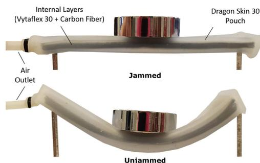
**FIGURE 2.** The soft laminar jamming structure can achieve multiple stiffnesses by applying a pressure gradient into the system. The structure is composed of a soft pouch made out of silicone rubber (Smooth-On Dragon Skin 30), an air outlet, and several thin layers made out of a combination of carbon fiber and silicon rubber (Smooth-On Vytaflex 30). When the vacuum is applied inside the pouch, the high friction between layers stiffens the entire structure.
