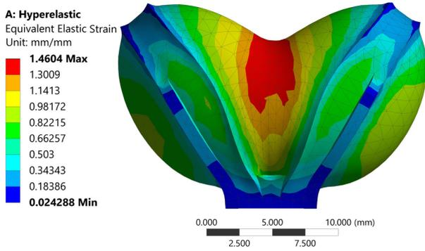
**FIGURE 6.** FEM analysis of the soft actuator employed for the execution of the abduction motion of the fingers at a pressure of 70 kPa. The maximum strain takes place in the interface between the two lateral walls of the actuator.
